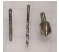
Countersink, for a better fit. Optional 8-32 drill and tap set
